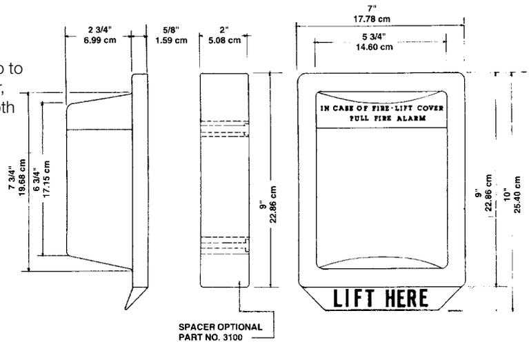
**NOTE:** If additional depth is needed, use the Conduit Spacer (Part No. STI 3100) which adds 2 inches (51mm) to the depth.
